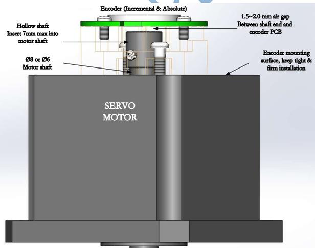
After coupling the encoder hollow shaft with the rigid motor shaft, always fasten attached screws securely. Be sure to firmly tighten two hex-screws that located at encoder's hollow shaft, apply threads-lock glue and tightly screwed in for long-term use. Also follow above procedures for the encoder M3 screws when mounting the encoder onto servo motor.
