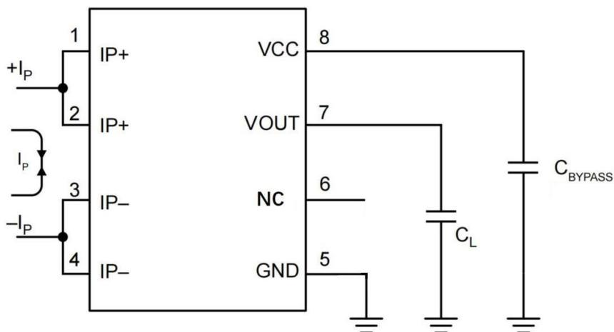
\* $C_{BYPASS}$  The capacitance needs to be placed close to the  $V_{CC}$  sensor
